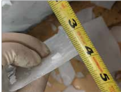
The Night Scan Powerlite IQ was tested at -15° F (-26° C) with a 1/4" (6mm) of ice
