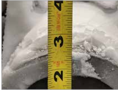
The Night Scan Powerlite IQ was tested at -15° F (-26° C) with a 1/4" (6mm) of ice
