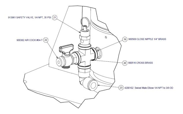
4. Ensure all items have been properly installed before returning your NS HDT Vertical light tower to service.
