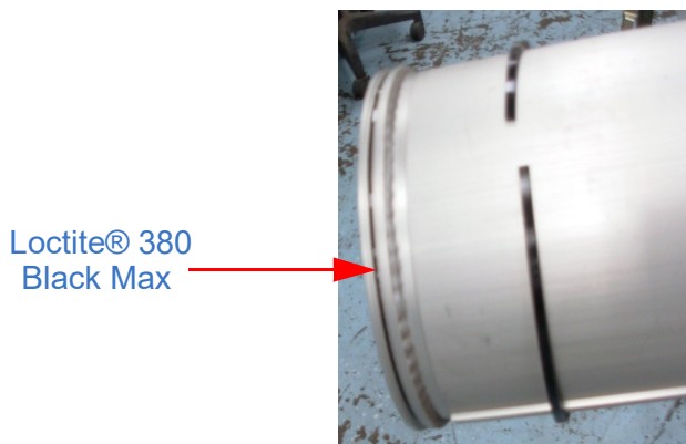
Figure 8-13 Loctite® 380 Black Max in Groove
