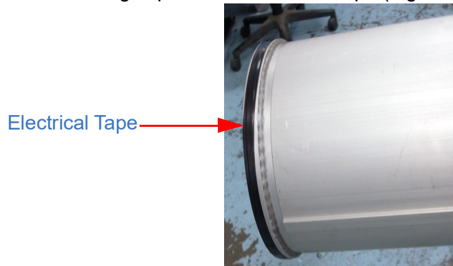
Figure 8-15 Electrical Tape Securing Wear Ring
