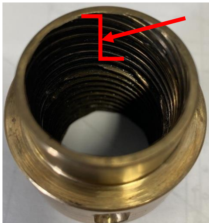
Over 25% Of Threads Worn or Missing
