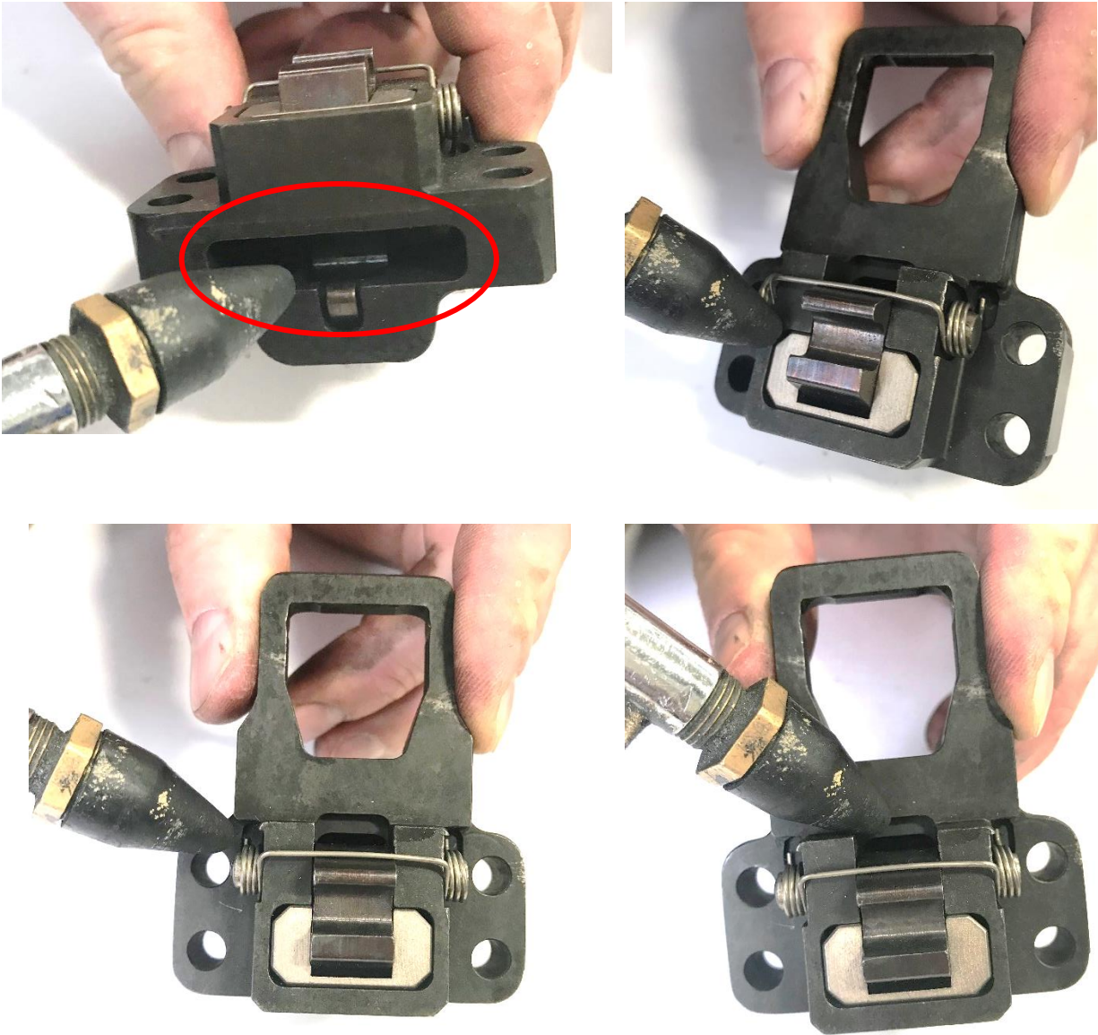
Figure 12 Blow Out Excessive Debris
