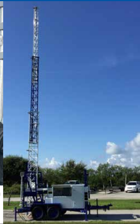
Patented Radial Slide Bar System Increases tower stability by reducing tower section movement when deployed
