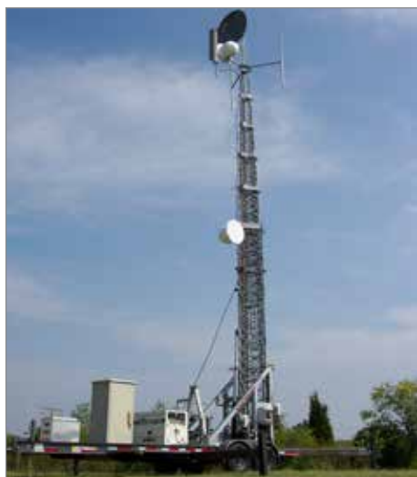
Steel Telescoping Tower Integrated Trailer System
