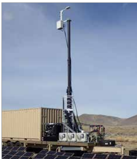
Telescoping Pneumatic Mast Integrated Trailer System
