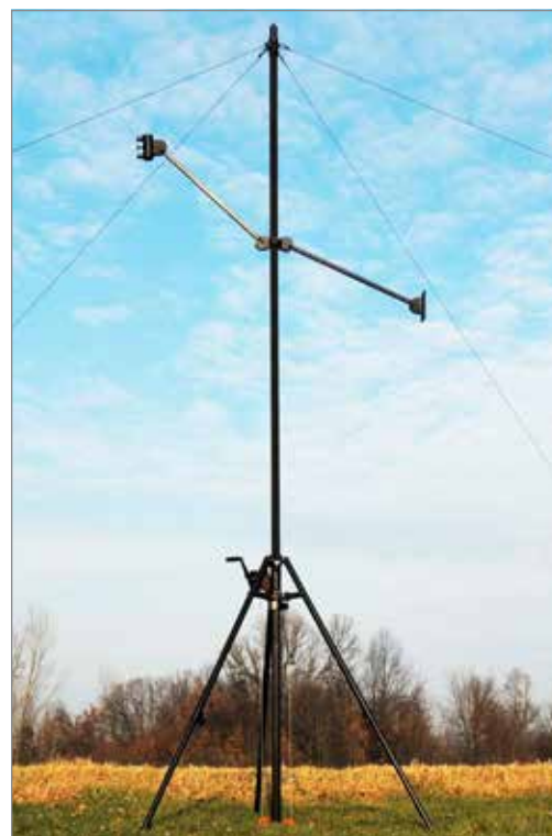
AM2 with Mast Tube Lift Winch
