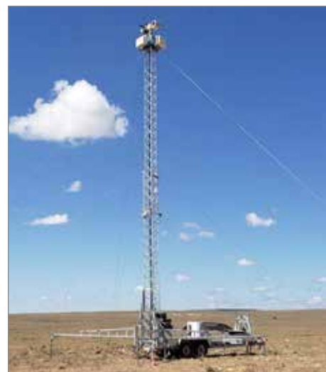
Aluminum Telescoping Tower Integrated Trailer System
