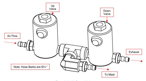
Figure 2-20 Air Control Valve
