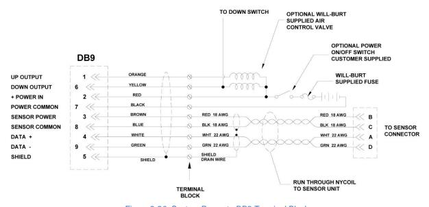
Figure 2-26 System Power to DB9 Terminal Block
