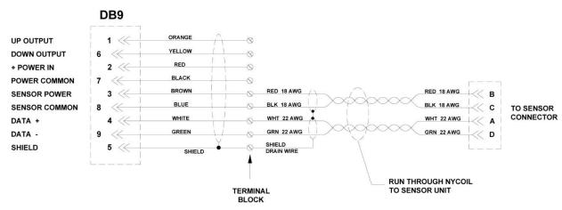
Figure 2-19 Sensor to DB9 Terminal Block
