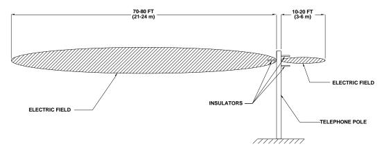
Figure 6-3 Electric Field Pattern
