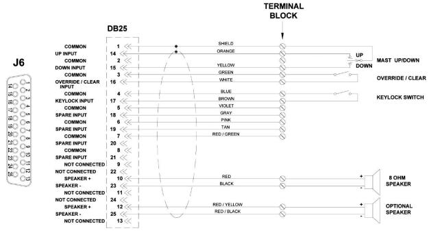
Figure 2-16 Install the Speaker
