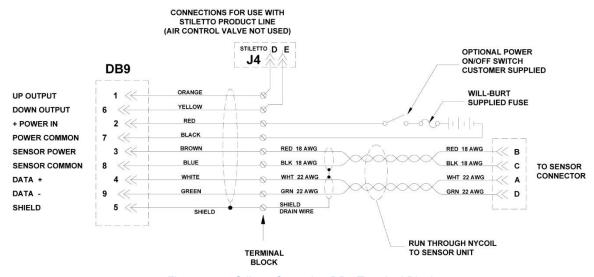
Figure 2-23 Stiletto Control to DB9 Terminal Block
