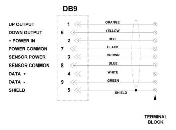
Figure 2-18 DB9 to Terminal Block
