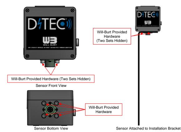
Figure 2-7 Mount Sensor to Installation Bracket
