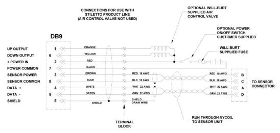
Figure 2-21 Air Control Valve to DB9 Terminal Block (Note: power not hooked up yet)
