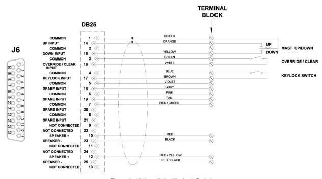
Figure 2-15 Install the Keylock Switch
