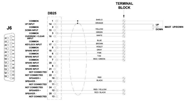
Figure 2-13 Install the Up/Down Switch
