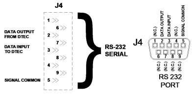
Figure 2-25 J4 Wiring
