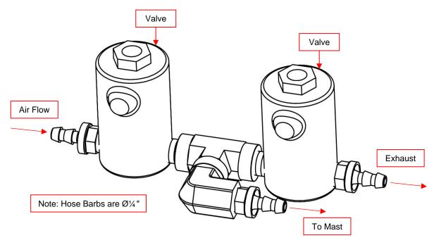
Figure 1-5 Air Control Valve
