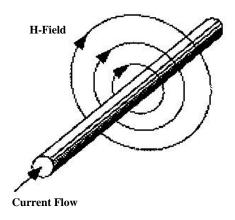
Figure 6-5 Magnetic Field Pattern
