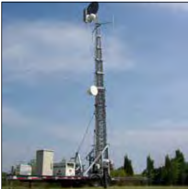
Steel Telescoping Tower Integrated Trailer System
