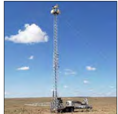
Aluminum Telescoping Tower Integrated Trailer System
