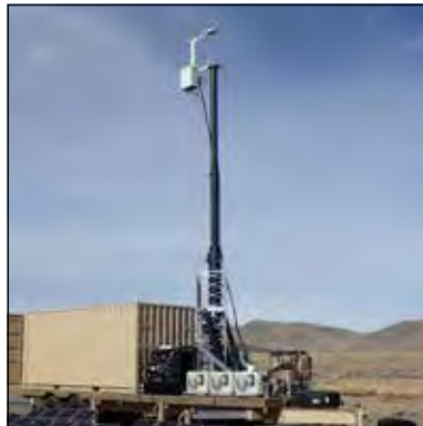
Telescoping Pneumatic Mast Integrated Trailer System
