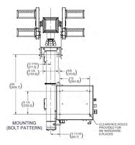
Figure 5-4 Night Scan Vertical Complete Mounting Hole Locations (Control Box Mounted to the Side of the Mast)
