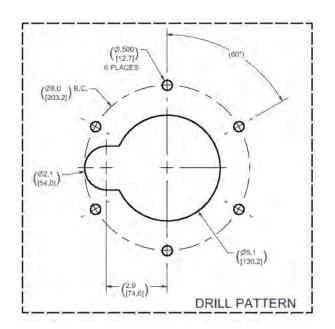
Figure 5-5 Internal Mounting Kit Roof Cutout Dimensions
