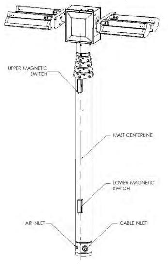
Figure 5-20 Upper and Lower Magnetic Switches
