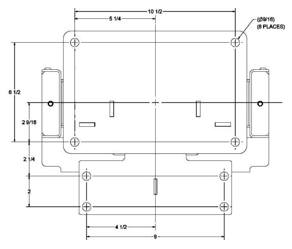
Figure 5-13 Night Scan Vertical HDT Saddle Mounting Holes
