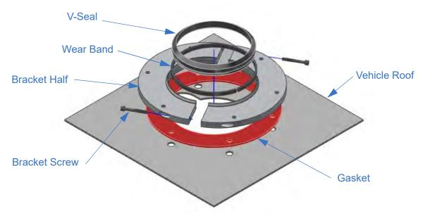
Figure 5-6 Internal Mounting Kit Assembly Detail
