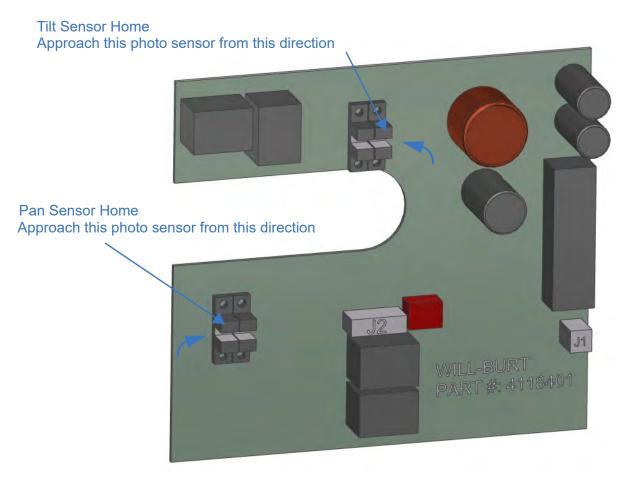
Figure 7-5 RCP PCB Photo Sensors
