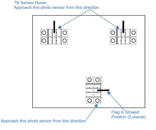
Figure 7-7 RCP PCB Photo Sensors (Dual-Tilt)
