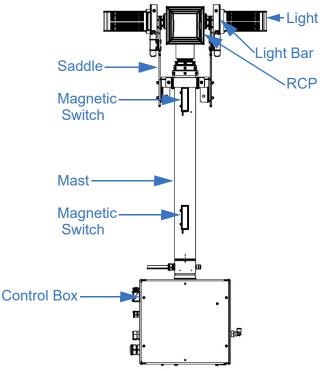
Note: Depending on the model, the control box may be attached either to the bottom or the side of the Night Scan Vertical Complete.
