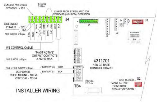
Figure 5-25 Wiring J4
