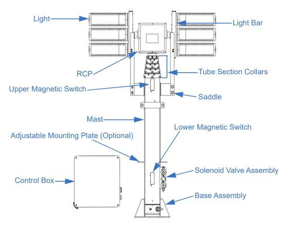
Figure 3-4 Night Scan Vertical HDT (Model 72030005 shown)
