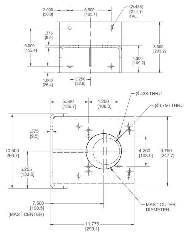
Figure 5-9 Shelf Bracket Installation Dimensions
