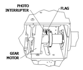
Figure 7-6 Dual-Tilt Photo Interrupter and Flag (cover removed)
