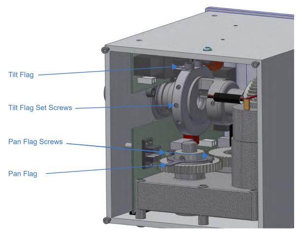
Figure 7-4 RCP Flags Single-Tilt RCP (cover removed)
