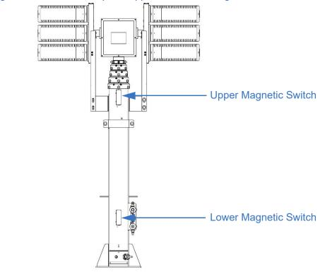
Figure 7-3 Night Scan Vertical Heavy Duty Towing (HDT) Upper and Lower Magnetic Switches
