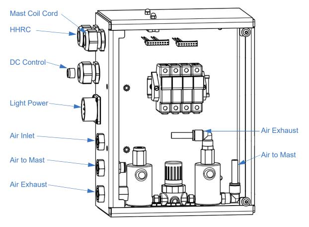
Figure 5-16 Control Box Valve Layout (Cover Removed)
