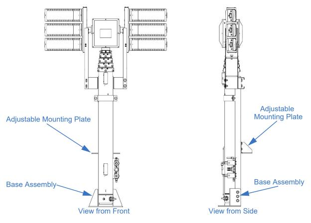
Figure 3-15 Night Scan Vertical HDT Mounting
