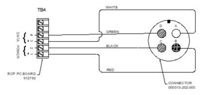
Figure 8-3 D-TEC® Wiring Schematic
