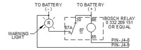
Figure 5-26 Example Vehicle Safety Interconnect Circuit
