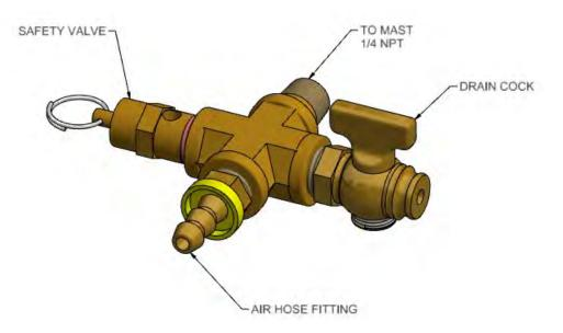
Figure 5-17 Mast Air Inlet Hardware Kit Assembly Detail
