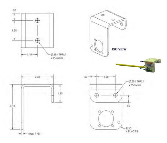
Figure 5-22 HHRC Bulkhead Bracket Installation Dimensions
