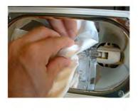
3. Obtain a napkin or towel free from debris, dirt, oil, etc. to remove the lamp.
