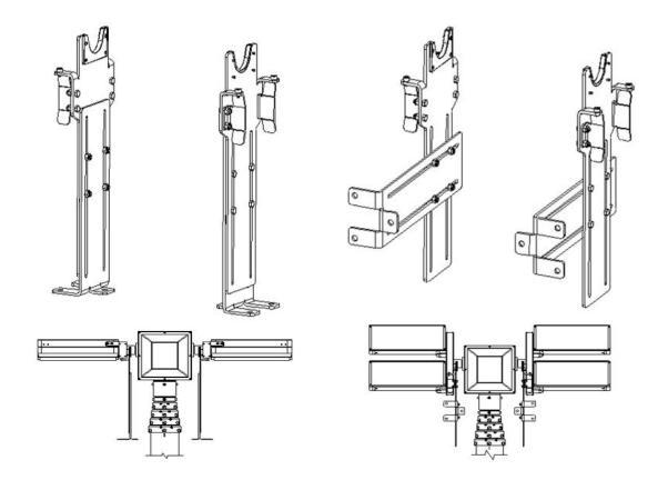
Figure 5-12 Mounting Variations. Clockwise from upper left: Saddle Deck Mount; Saddle Wall Mount; Saddle and RCP Assembly Lights Stowed Horizontally; Saddle and RCP Lights Stowed Vertically
