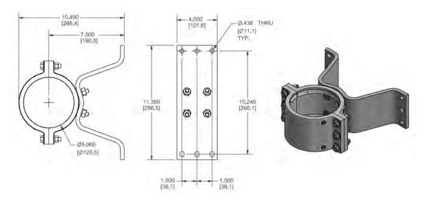
Figure 5-8 Support Bracket Mounting Dimensions
