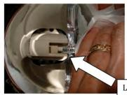
4. Holding the lamp with the napkin, push in as far as possible on spring-loaded lamp holder on the left. This should release or free the lamp for removal (see step #5)
