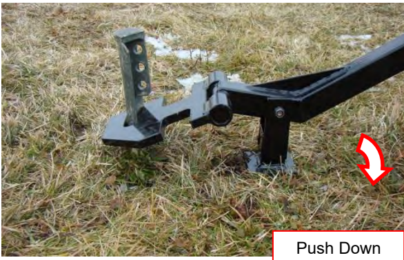
Figure 5-18 Push Down on Stake Puller Handle
