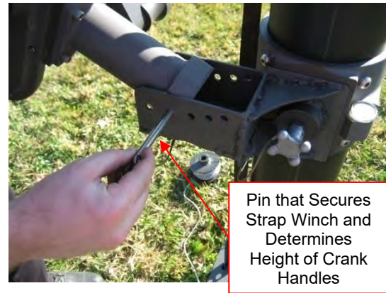
Figure 4-23 Secure Winch at Desired Position
