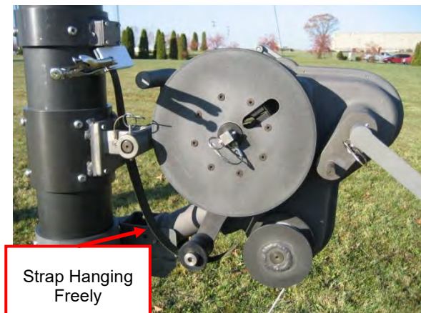
Figure 8-2 Crank Winch in Reverse Direction
