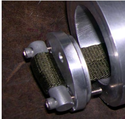
Figure 7-10 Secure Strap Pin in Place
