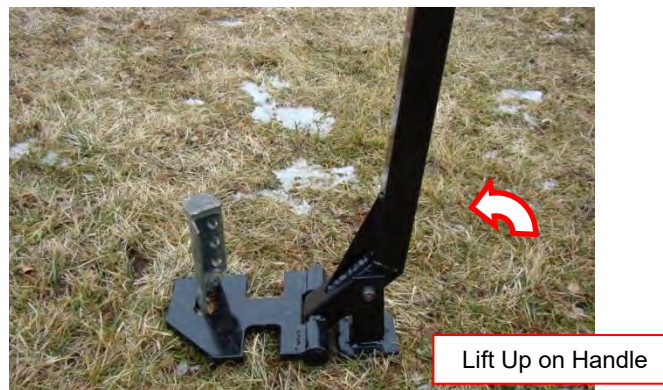
Figure 5-19 Lift Up on Handle
