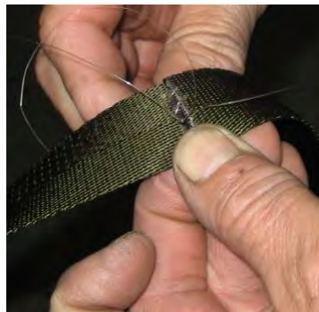
Figure 7-3 Create a Butt Splice
