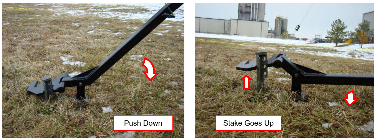
Figure 5-16 Push Down on Stake Puller Handle
