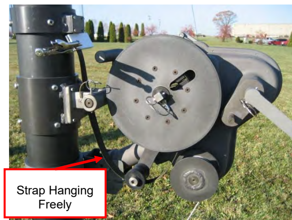
Figure 8-4 Crank Winch in Reverse Direction to Transfer Load from Winch to Clamp Block
