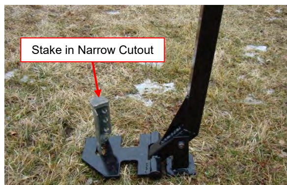
Figure 5-17 Place Narrow Cutout Over the Stake
