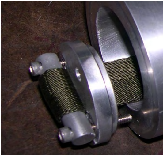
Figure 7-8 Pull Out the Top Stub Cap
