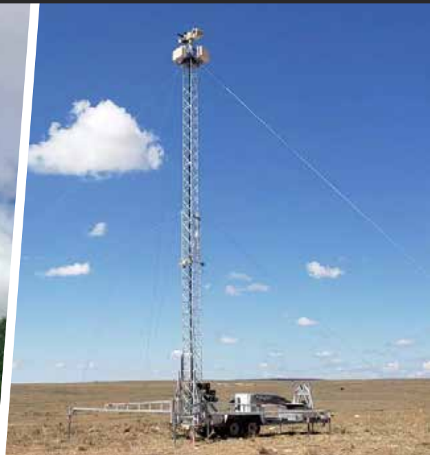
Aluminum Telescoping Tower Integrated Trailer System
