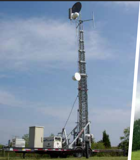
Steel Telescoping Tower Integrated Trailer System
