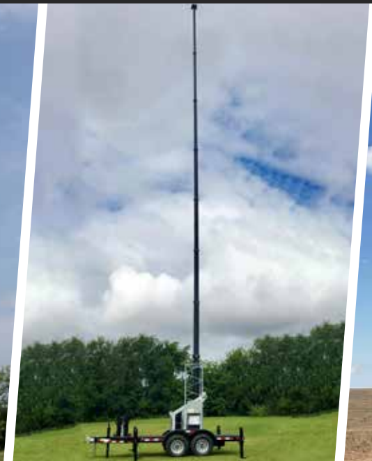
Telescoping Pneumatic Mast Integrated Trailer System
