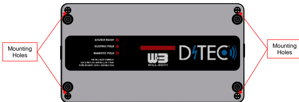
Figure 2-9 Wall Mount Display Mounting Hole Locations
