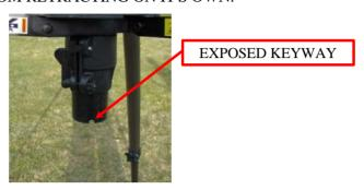
2 PLACE THE NEXT TUBE TO BE LOADED UNDER THE BOTTOM CLAMP OF THE TRIPOD (CURRENTLY LOCKED). ALIGN THE KEY OF THE TUBE BEING LOADED WITH THE KEYWAY OF THE TUBE LOCKED IN THE LOWER CLAMP. BE SURE THE KEY AND THE KEYWAY ARE ALIGNED/MATED PROPERLY IN ORDER TO ENSURE PROPER DEPLOYMENT OF THE MAST AS WELL AS PREVENT THE KEYS FROM BEING SHEARED UNDER THE WEIGHT OF THE MAST/PAYLOAD (IF NOT IN PLACE AS DESCRIBED).
