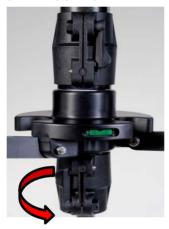
B INSERT THE TOP MAST SECTION FROM THE TOP AND SECURE IN PLACE (AT A COMFORTABLE WORKING HEIGHT) BY LOCKING THE LOWER CLAMP ON THE TUBE. THE TOP SECTION CAN BE IDENTIFIED AS THE SHORTEST OF ALL OF THE MAST SECTIONS.
