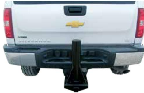
Figure 4-3 Secure Hitch Mount to Vehicle
