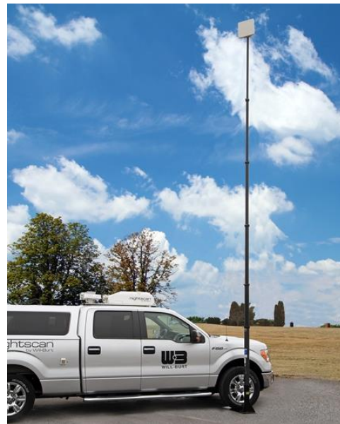
Figure 4-2 Mast Mounted with Drive-On Stand
