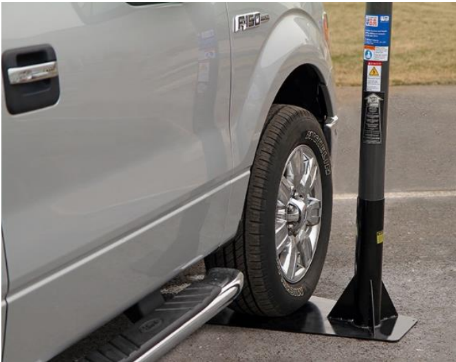
Figure 4-2 Mast Mounted with Drive-On Stand
